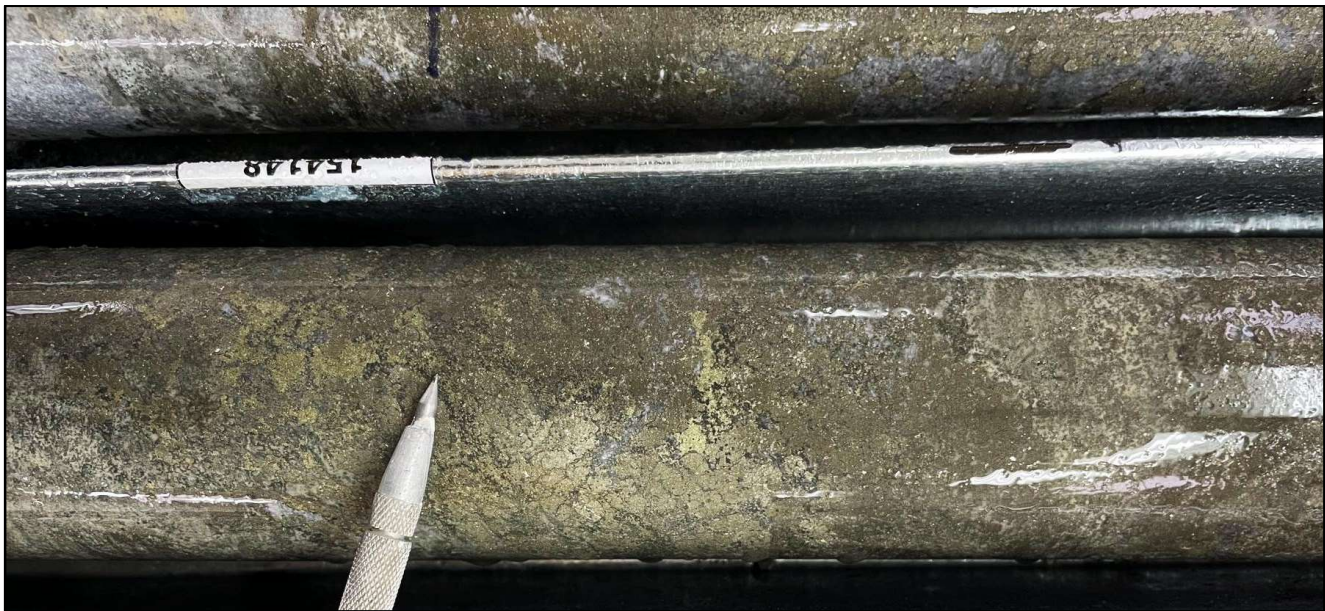
Figure 8. Core photo of semi-massive sulphides with gold-copper-zinc mineralisation from 248.8m in ZRSD24154 – 1.3g/t Au, 0.5% Cu and 0.2% Zn.
