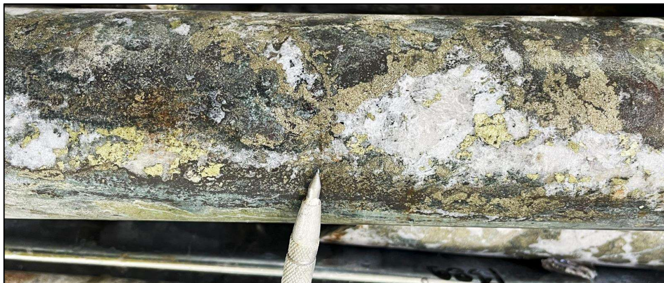
Figure 1. Core photo of copper-gold-mineralisation from 388.5m in ZRSD24153 – 0.8g/t Au and 0.9% Cu.
