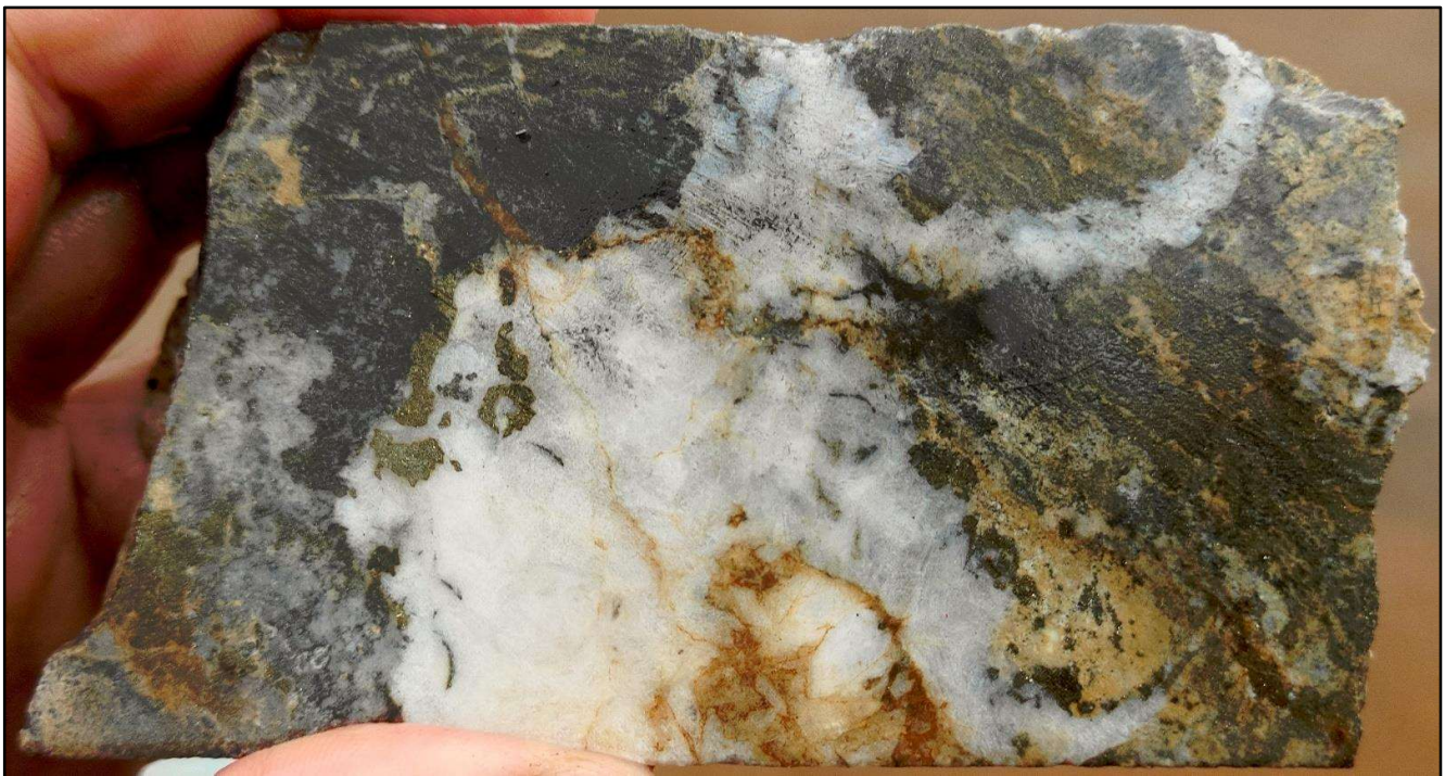
Figure 6. Gold-only mineralisation associated with quartz-carbonate veining in endoskarn from 595.5m downhole depth in ZRSD24163 – 5.3g/t Au.
