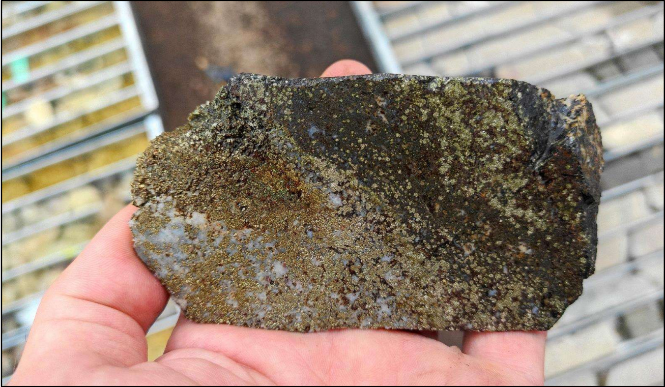
Figure 5. Photo of gold-copper-zinc mineralisation from 278m down-hole depth – 2.1g/t Au, 0.4% Cu, 2.6% Zn and 9.6g/t Ag.
