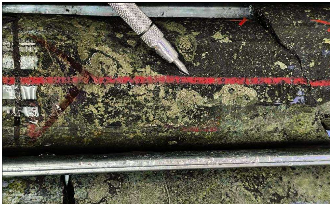
Figure 7. Core photo of semi-massive sulphides with gold-copper-silver mineralisation from 371.1m in ZRSD24160 – 4.4g/t Au, 4.3% Cu and 49.8g/t Ag (12.8g/t AuEq).
