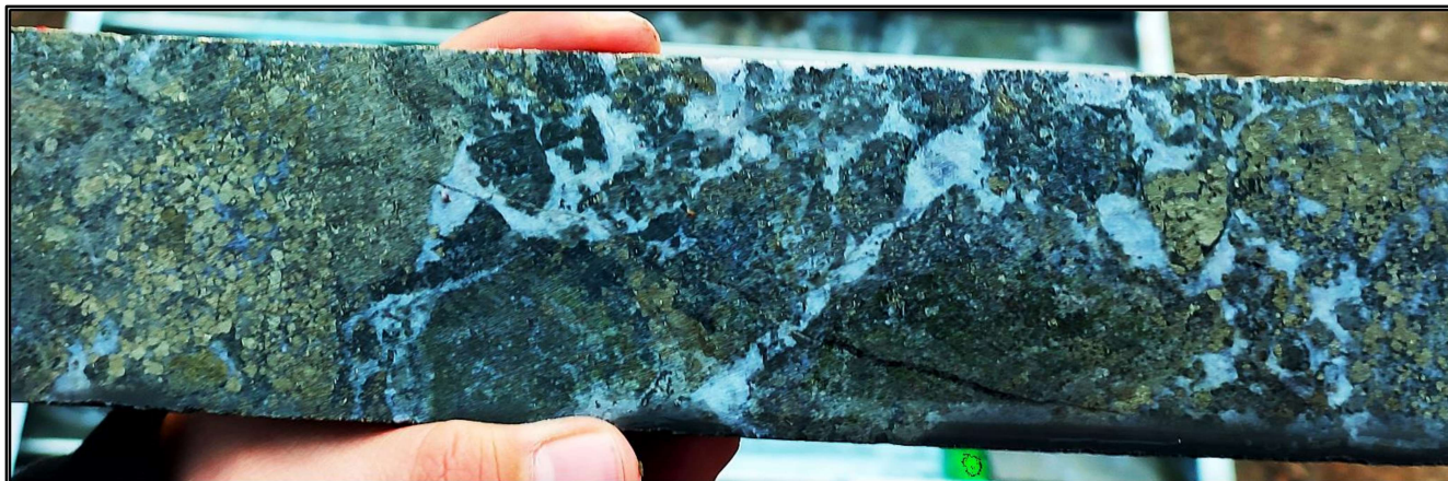
Figure 6. Core photo of pyrite-rich gold mineralisation from 267.3m in ZRSD24167– 4.2g/t Au.
