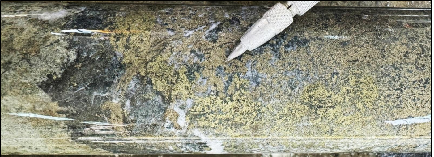
Figure 8: Core photo of skarn-hosted mineralisation with semi-massive chalcopyrite and pyrite from 603.0m in ZRSD25176 – 5.1g/t Au, 1.6% Cu and 14.9g/t Ag (7.5g/t AuEq 2 ).
