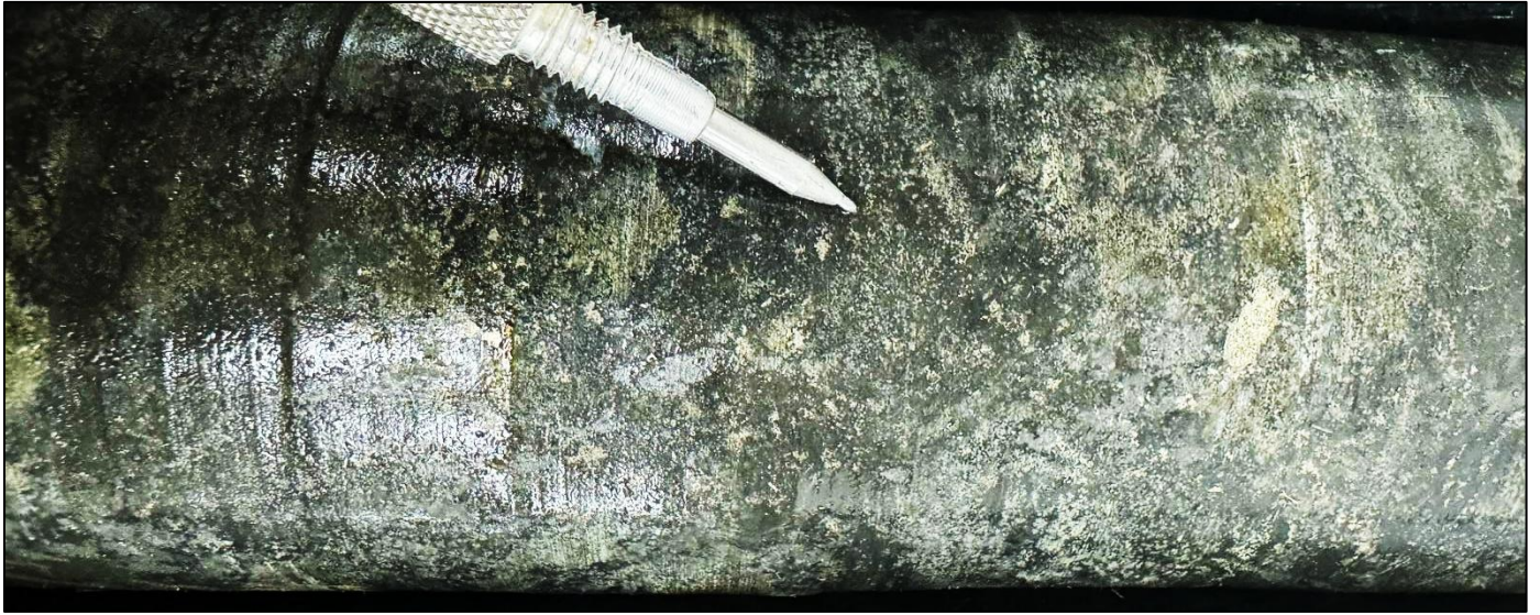
Figure 6: Core photo of magnetite skarn with magnetite, chalcopyrite, sphalerite and pyrite from 485.9m in ZRSD25175 – 2.6g/t Au, 0.9% Cu, 0.4% Pb, 1.0% Zn and 34.2g/t Ag (4.8g/t AuEq 2 ).
