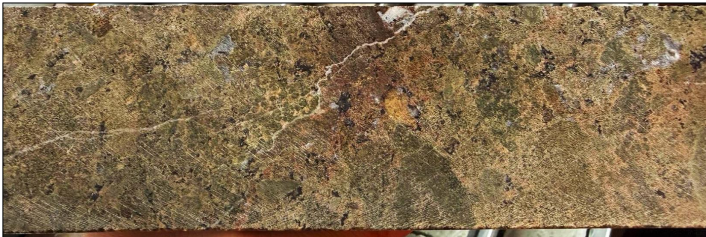
Figure 5. Core photograph from 537.5m to 539.5m in ZRSD25212 showing strong pyrite, sphalerite and arsenopyrite mineralisation – 12.1g/t Au, 0.9% Zn and 0.8g/t Ag.
