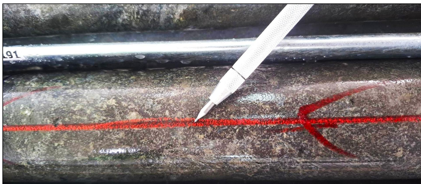
Figure 6. Core photograph from 333.7 to 335.7m in ZRSD25220 showing pyrite and sphalerite mineralisation – 4.3g/t Au, 8.9% Zn and 1.0g/t Ag.
