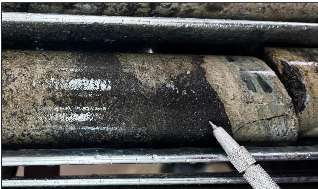
Figure 7. Core photograph of ZRSD25239 from 516.8 to 518.8m showing semi-massive sphalerite-pyrite-magnetite – 4.8% Zn.
